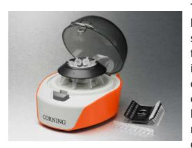
The Corning LSE Mini Microcentrifuge is a personal bench top instrument that operates at a fixed speed of 6,000 rpm (2,000 x g) and was designed for quick spin downs of micro-samples. Operation is made simpler and more convenient with the design of a quick-release rotor system and electronic brake. Once samples are loaded and the lid is closed, the rotor rapidly accelerates to 6,000 rpm. This speed range is ideal for bringing small droplets to the bottom of the tubes for
