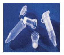
Spin-X centrifuge tube filters consist of a membrane-containing (either cellulose acetate or nylon) filter unit within a polypropylene centrifuge tube. They filter small sample volumes by centrifugation for bacteria removal, particle removal, HPLC sample preparation, removal of cells from media and purification of DNA from agarose and polyacrylamide gels
