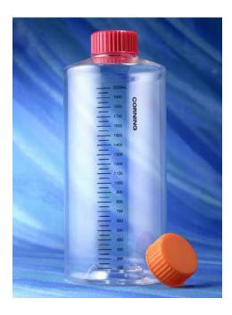
Ideal for a variety of rolling applications, Corning Roller Bottles are made of USP Class VI Polystyrene. They are single-use, sterile, feature laser-etched graduations, and are available in 490 cm², 850 cm², 1700 cm² pleated, and 1750 cm² sizes. Caps are available in solid High Density Polyethylene (HDPE) or vented HDPE with a 0.2 mm micro-porous PTFE membrane.
