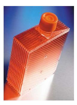
The Corning High Yielding Performance Flask (HYPERFlask) cell culture vessel offers a 1720 cm<sup>2</sup> growth area in the footprint of a traditional 175 cm<sup>2</sup> flask. This high yield, high performance flask utilizes a multilayered gas permeable growing surface for efficient gas exchange.
