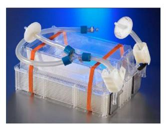
Closed System for High Yield Cell Growth: Introducing the next generation in Corning's High Yield PERformance the (HYPER) platform \_ Corning HYPERStack cell culture vessel. This product line combines the best of two Corning products: the Corning CellSTACK® culture chamber and the Corning HYPERFlask® vessel. The utilization of the proprietary gas-permeable film technology provided in the format of the CellSTACK culture chamber allows the HYPERStack
