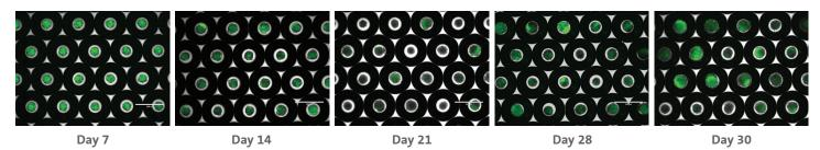
The Corning Elplasia 12K flask enables long-term cultures. A-549/GFP (human lung carcinoma) spheroids cultured in a Corning Elplasia 12K flask for 30 days. Micrographs were taken with an EVOS FL microscope in brightfield and GFP modes using a 2X objective.
