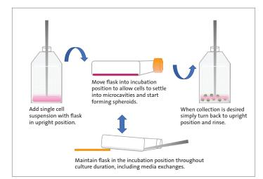
The Corning<sup>®</sup> Elplasia<sup>®</sup> 12K flask was designed to enable the generation of a large volume of uniform spheroids under one culture condition with a simple "plug and play" protocol. For more details, please refer to the Corning Elplasia 12K flask Guidelines for Use (CLS-AN-713DOC).
